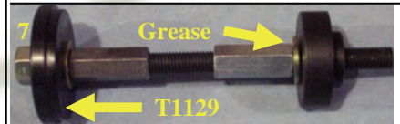
TS4643 Inner Axle Seal Installer for Super Duty Dana 50 front axles. This tool will also work on Super Duty Dana 60 axles if you replace T1129 Thrust Plate with T1130.
