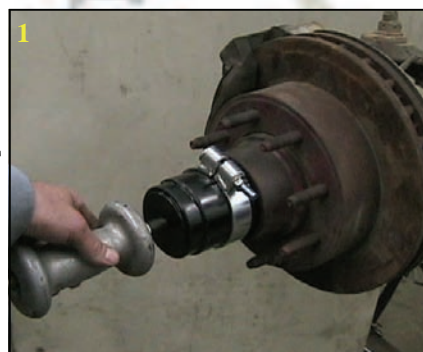
Removing a stuck Stock Lockout Hub with T1124 Puller and QT9302 Slide Hammer
